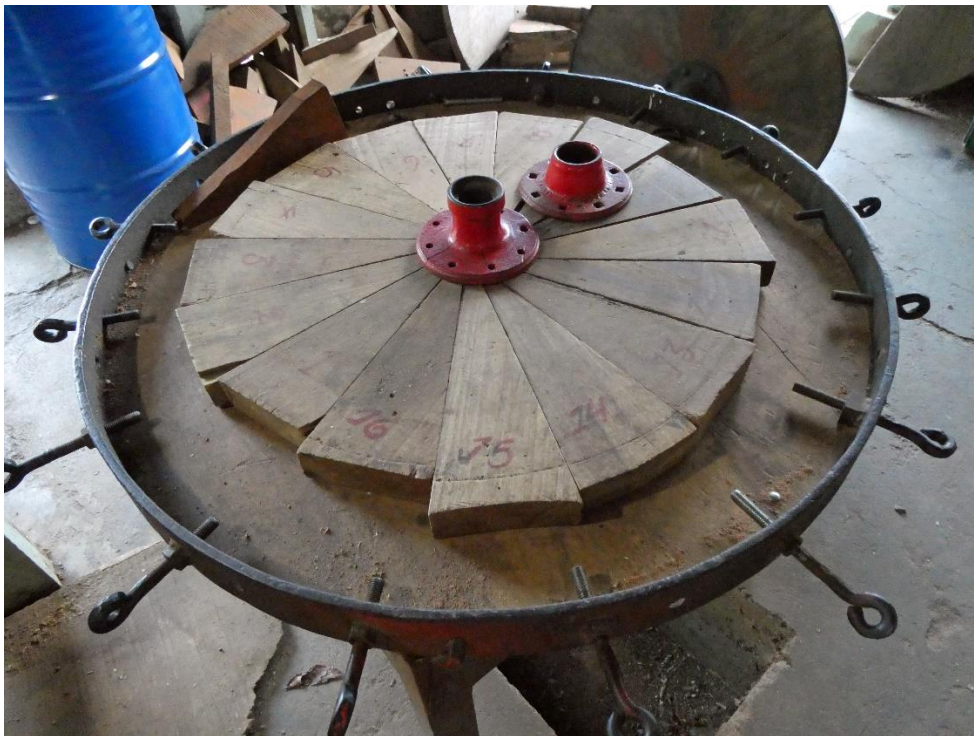
A traditional oxcart wheel in progress, using traditional manufacturing techniques. Once the wood segments are properly trimmed, an iron rim will be fitted around them. The equipment in the manufacturing shop is still powered by a water wheel.
