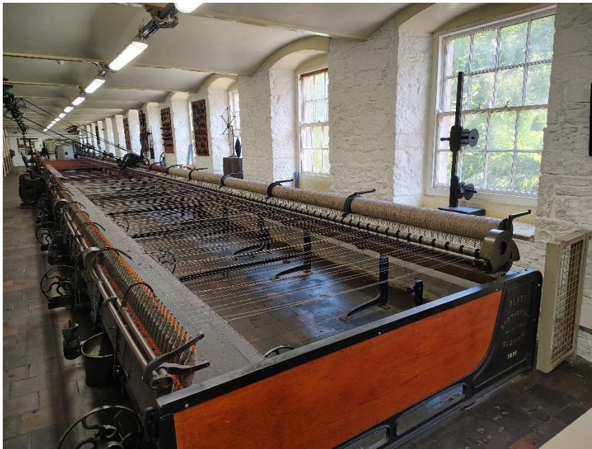
Large weaving looms were powered by water from the River Clyde.
